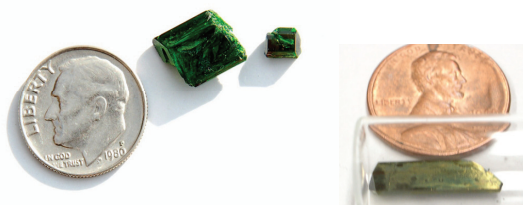
FIGURE D.2 (Left) Crystals of \text{Ni}_2\text{SiO}_4 olivine grown from an \text{Na}_2\text{MoO}_4\text{-Li}_2\text{MoO}_4\text{-NaCl} solution after cooling for a month. SOURCE: Courtesy of Robert J. Cava, Princeton University. (Right) Methyl pyridium tetracyanoethenide grown from acetonitrile after cooling for 4 days. SOURCE: From J.S. Miller, P.M.B. Piccoli, A.J. Schultz et al., CrystEngComm , 11 , 686-690 (2009). Reproduced by permission of the Royal Society of Chemistry.
