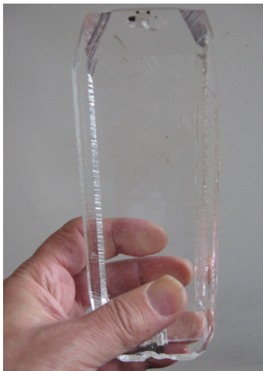
FIGURE D.4 A single hydrothermally grown quartz crystal. SOURCE: Courtesy of Robert J. Cava, Princeton University.
